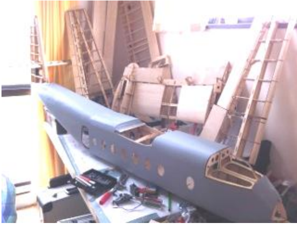
Fuse sheeted & primed
