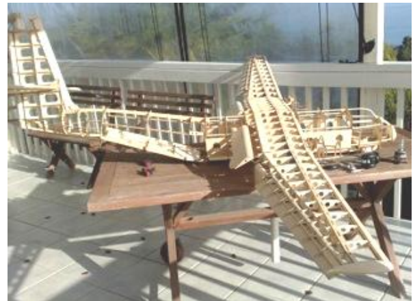
Ready for sheeting
